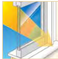
In warm weather, Low-E glass reflects the sun’s energy and reduces heat gain in the home.
